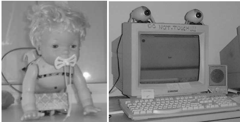
Figure 1. The first physical implementation of the robot baby has microphones in its ears, crude switches for touch, independent control of the head and each limb, and internal sensors for orientation and acceleration/shock. The electronics is controlled by a 6809HC11 microcontroller. Philips USB videocams are currently used externally for vision, and also provide additional microphones, but the next version will incorporate the cameras internally.
