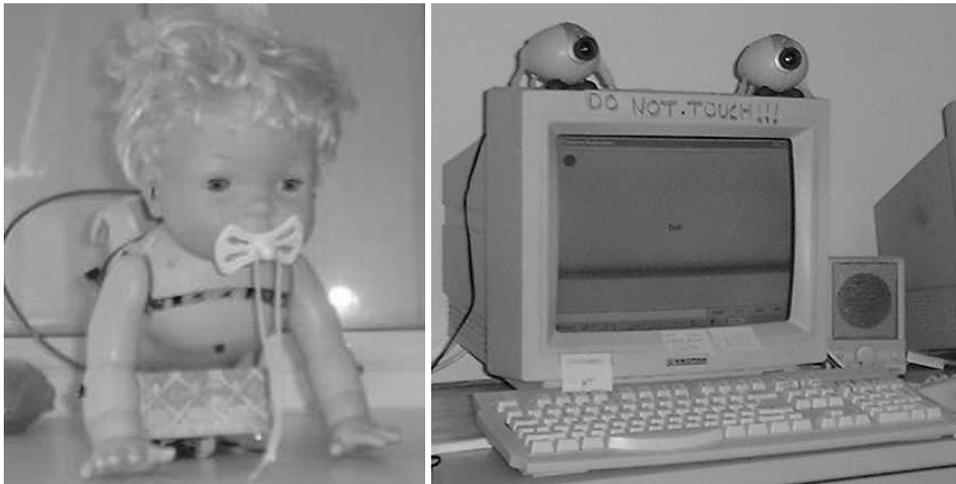
**Figure 1.** *The first physical implementation of the robot baby has microphones in its ears, crude switches for touch, independent control of the head and each limb, and internal sensors for orientation and acceleration/shock. The electronics is controlled by a 6809HC11 microcontroller. Philips USB videocams are currently used externally for vision, and also provide additional microphones, but the next version will incorporate the cameras internally.*
