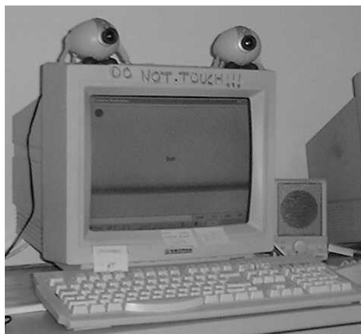
Figure 2. Philips USB videocams are currently used externally for vision.
