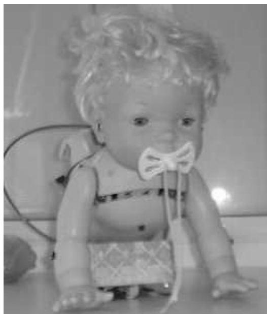
Figure 1. The first physical implementation of the robot baby has microphones in its ears, crude switches for touch, independent control of the head and each limb, and internal sensors for orientation and acceleration/shock. The electronics is controlled by a 6809HC11 microcontroller.
